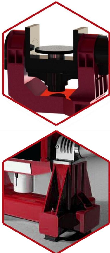
The two-axis turntable is a kind of precision test equipment, which can provide the angular position, angular rate and angular acceleration motion excitation of two orthogonal axes to realize the test and evaluation of the measured parts such as gyro, inertial measurement device and accelerometer, and can also realize the dynamic motion simulation, servo, simulation and angular vibration of the two rotation directions in space.
